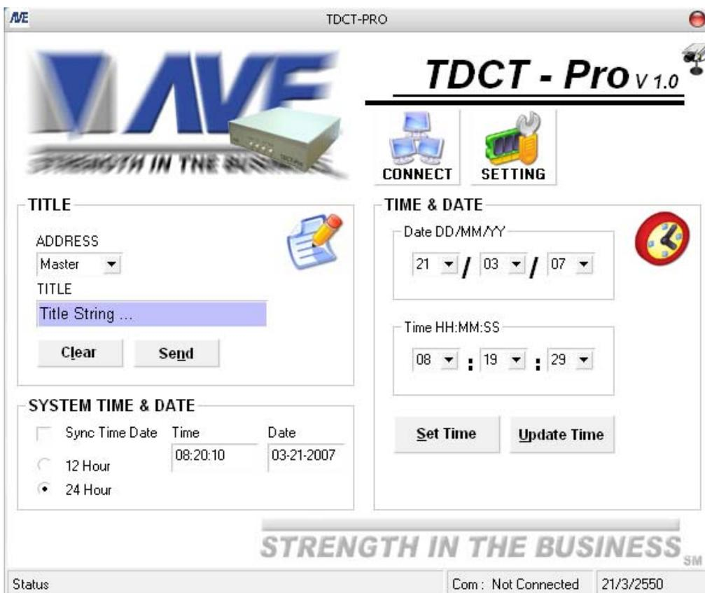
Click the “Setting” for set Comport, Baudrate, Data Bit, Parity Bit and Stop Bit.
